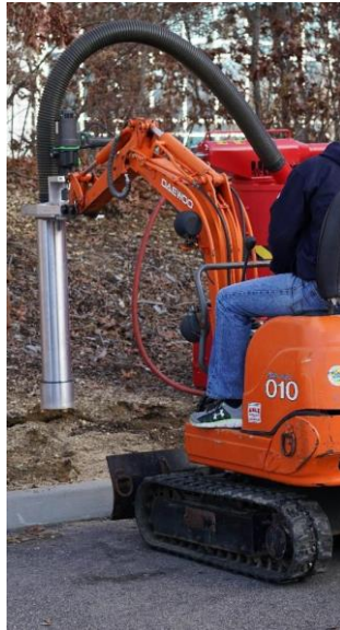
Figure 7 - Prototype 1, developed through the second phase of the project to prove the concept of soft-touch
